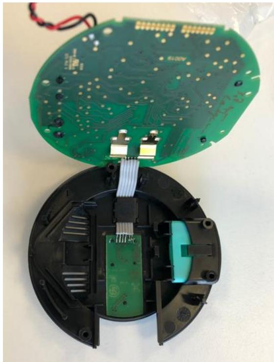
Inner part mounted completely except upper housing
