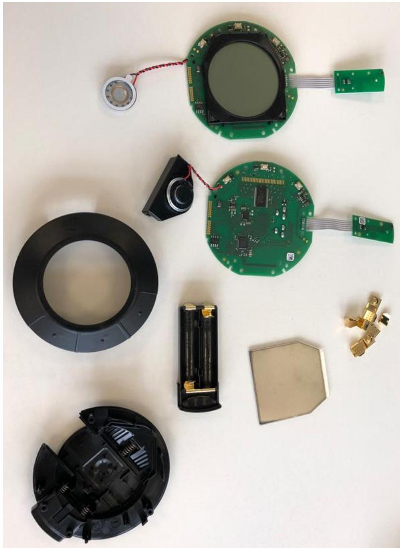
Magnetic sensor (small PCB) mounted in lower case, connected to the main PCB via flat cable
