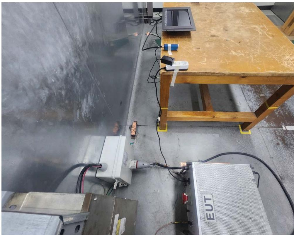
**[ Radiated Disturbance Test Set Up (Below 1 GHz) ]**
