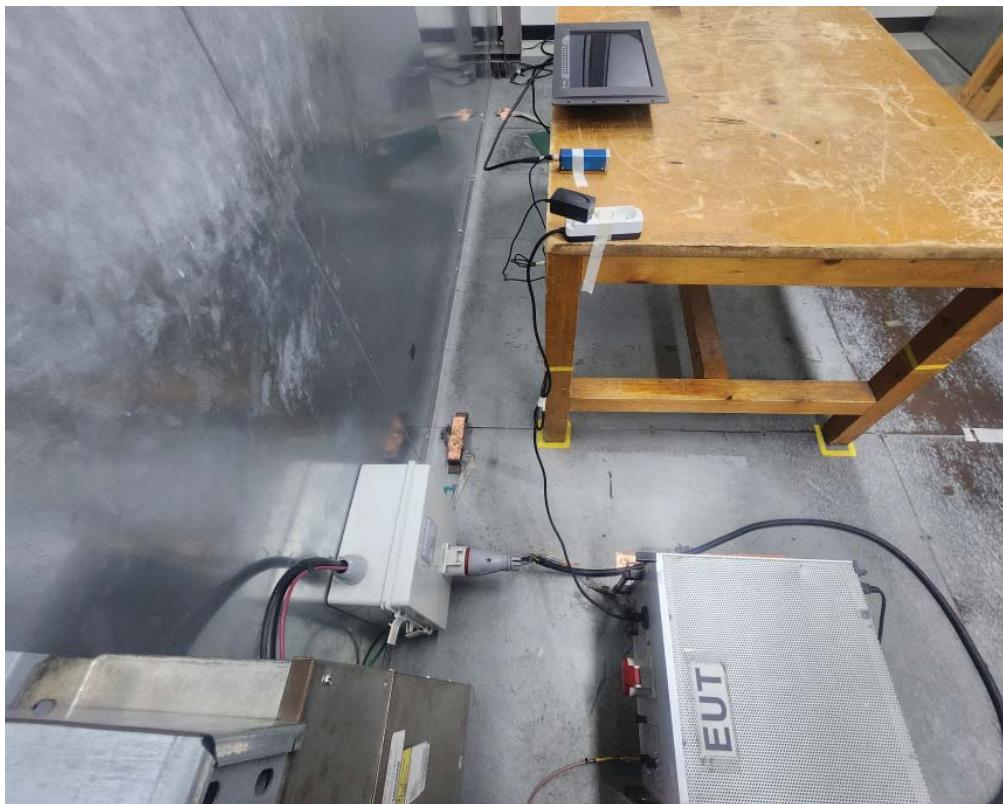
**[ Radiated Disturbance Test Set Up (Below 1 GHz) ]**
