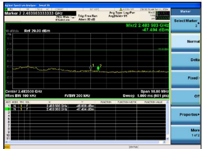
802.11b HIGH CHANNEL, BAND EDGE
