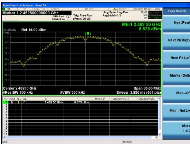
802.11b HIGH CHANNEL, CARRIER LEVEL
