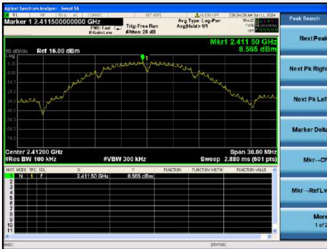
802.11b LOW CHANNEL, CARRIER LEVEL
