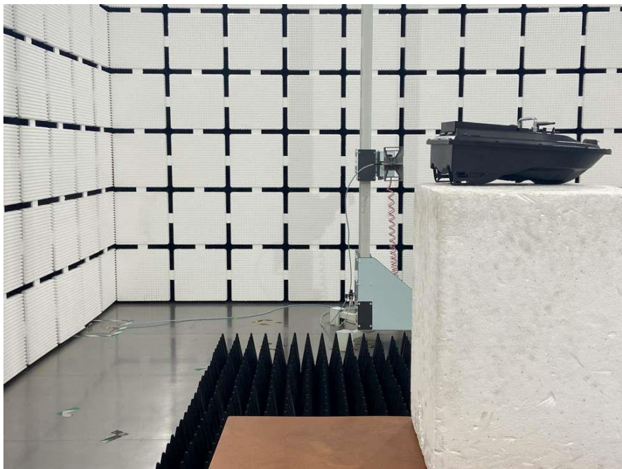
Radiated Emission Test View Above 1GHz
