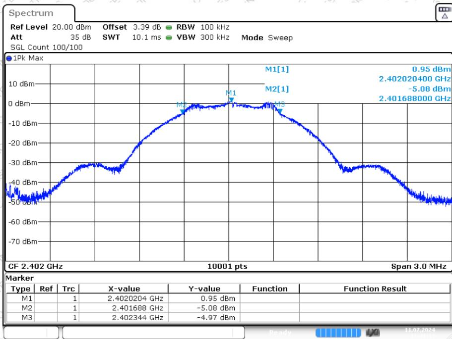
**-6dB Bandwidth NVNT BLE 1M 2440MHz Ant1**
