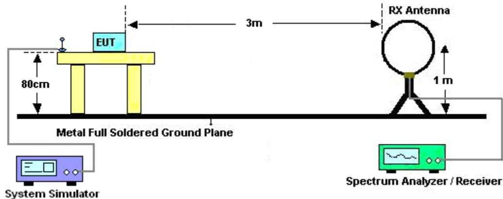
For radiated emissions from 30MHz to 1GHz
