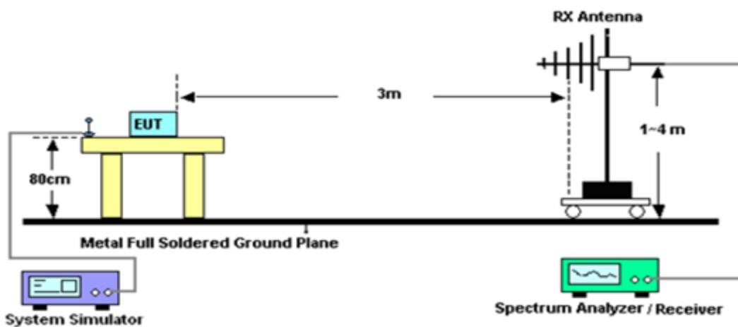
For radiated test above 1GHz
