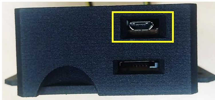
Figure 5 Catena4430 Micro USB Port Cutout
