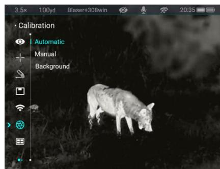
temperature of the detector and eliminate the image defects (such as vertical bars, phantom images, etc.).
