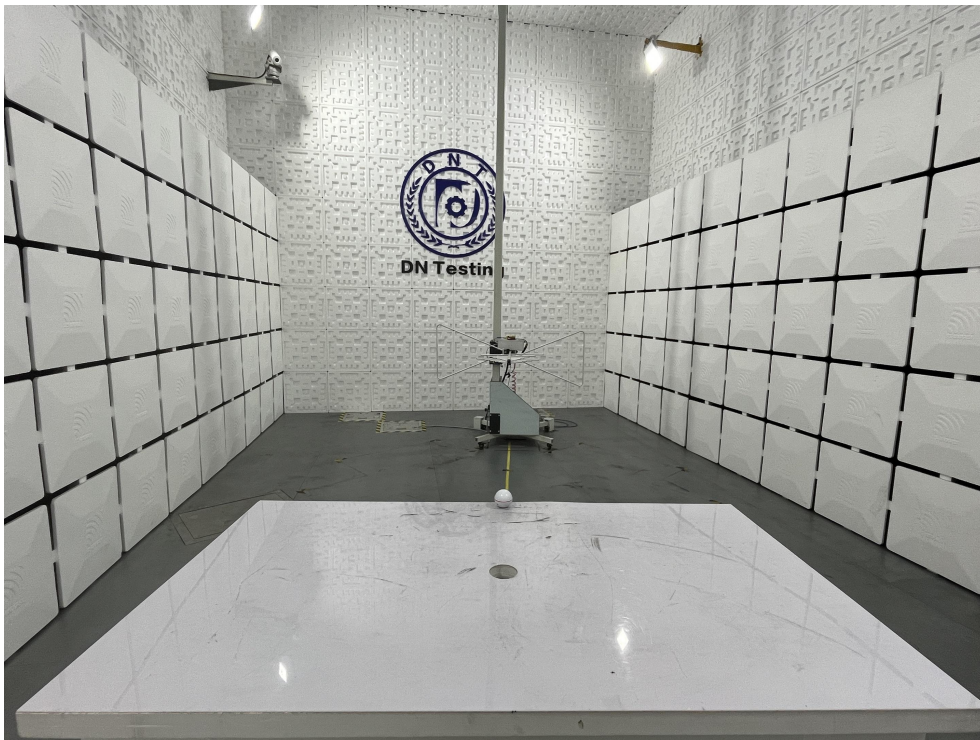
Radiated Emission Test View|(Below 1G)
