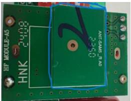
A photograph of the antenna module. It is a green printed circuit board (PCB) with various electronic components. A blue outline highlights a rectangular area in the center, which is the antenna itself. The PCB is labeled with 'HNK' and 'HF MODULE-A5' on the left, and 'ANT-SAM5' on the right. There are also some component designators like '2222' and '2223'. |
