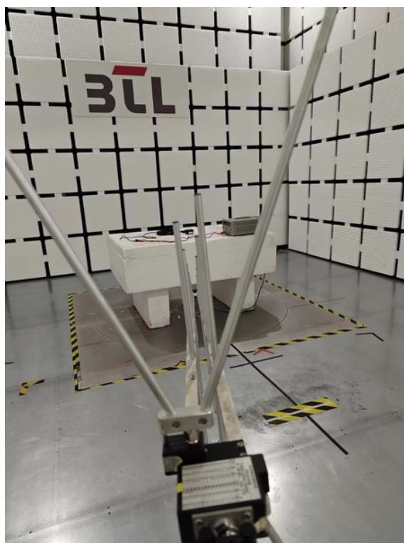
**Radiated Emissions Test Photos****Above 1 GHz**
