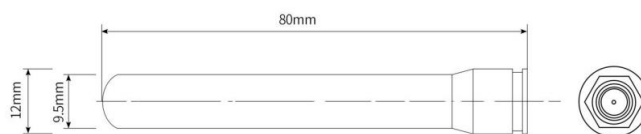
Figure 5 FCC: 915 MHz antenna dimensional drawing
