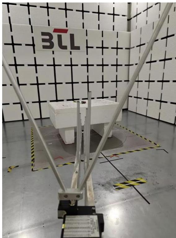
**Radiated Emissions Test Photos****Above 1 GHz**
