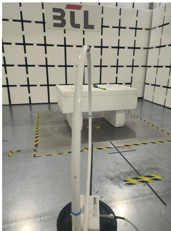
**Radiated Emissions Test Photos****30 MHz to 1000 MHz**
