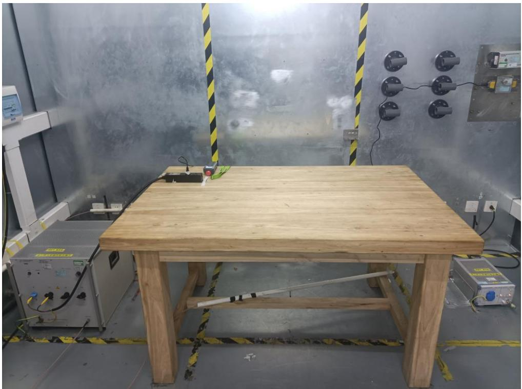
**Radiated Emissions Test Photos****9 kHz to 30 MHz**
