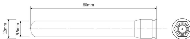
Figure 5 FCC: 915 MHz antenna dimensional drawing
