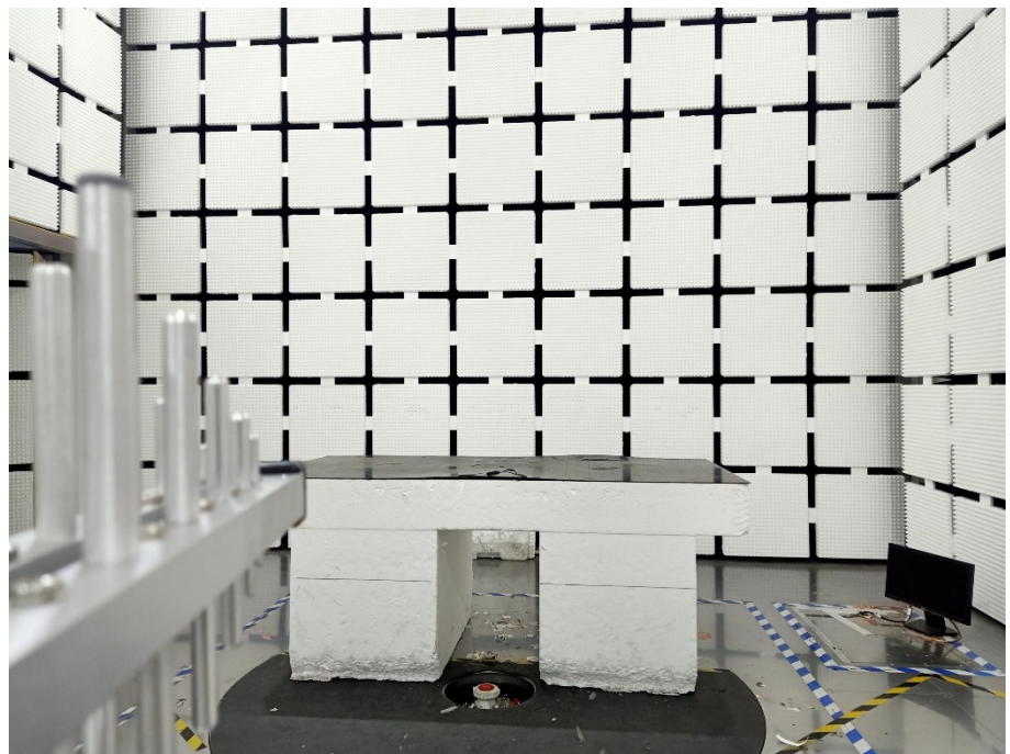
Radiation Emission Test Setup (30MHz to 1GHz)
