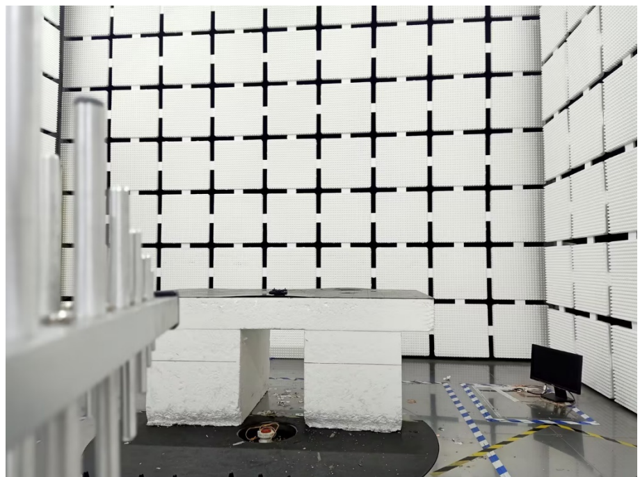
Radiation Emission Test Setup (30MHz to 1GHz)
