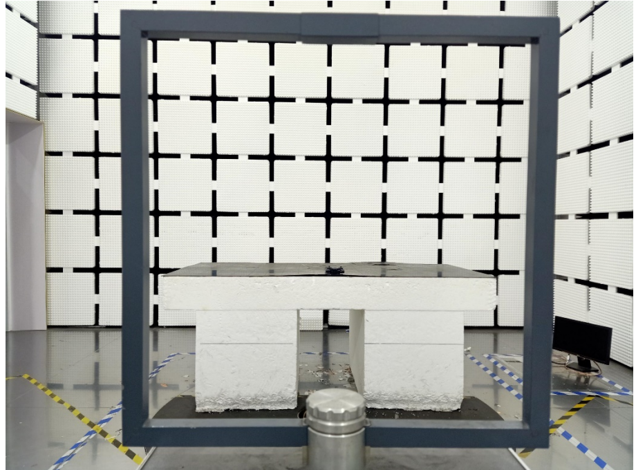
Radiation Emission Test Setup (Below 30MHz)
