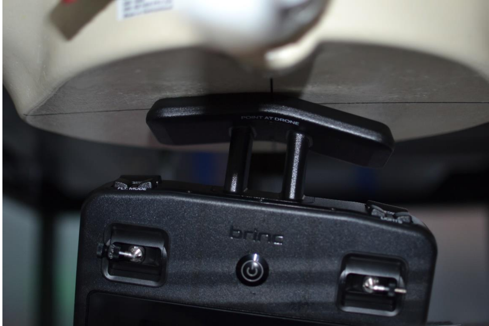
SAR Test Setup Photo 3 – Top Edge Ant A at 0mm
