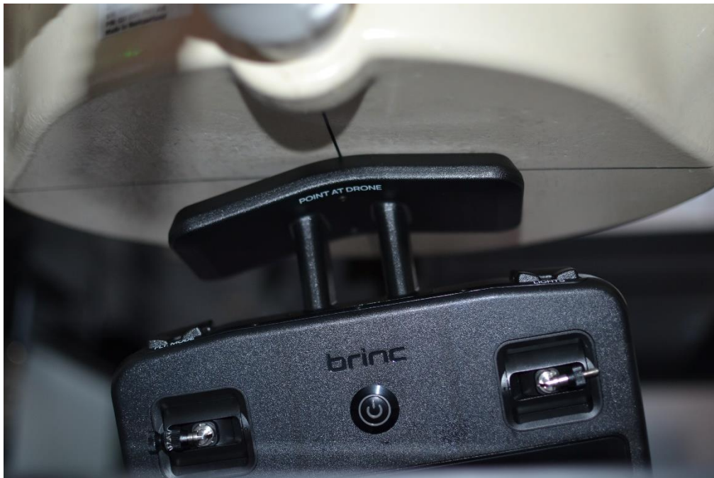
SAR Test Setup Photo 4 – Top Edge Ant B at 0mm
