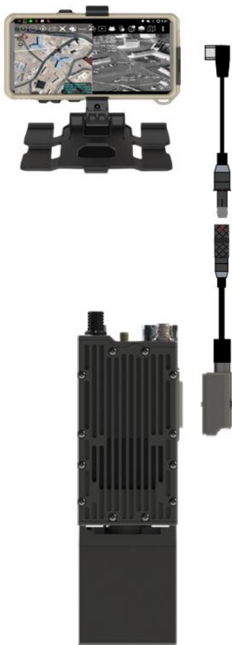
Figure 11-2 ATAK to SDR-H2 Connections
