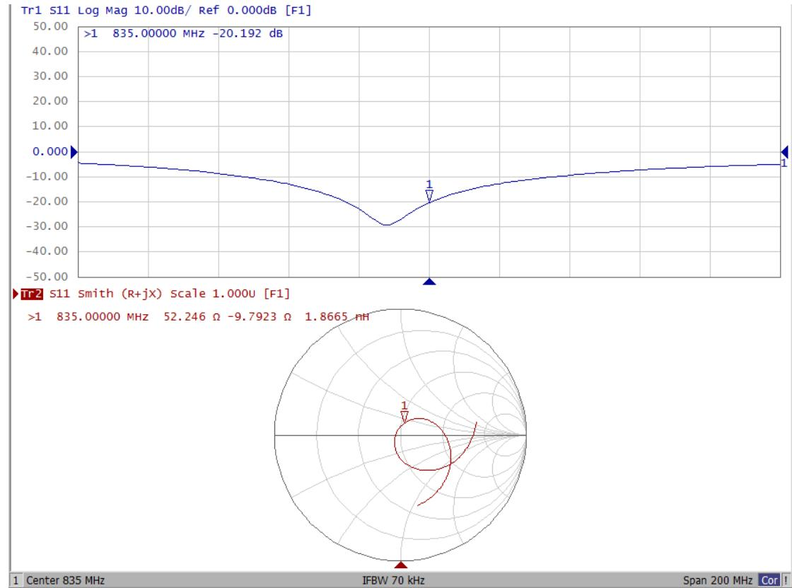
Dipole Verification Data > D835V2 - SN:453 (Date of Measurement: 2023/8/30)
