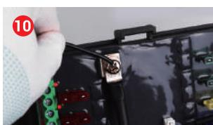
Connect light to control box, and negative wires can be connected to the **common cathode**
