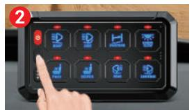
Then short press the brightness adjustment button. When the **blue backlight flashes**, it enters the Strobe setting state
