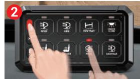
Press the button you want to set (you can choose between 8 or 12 buttons for Momentary Mode), then press the ON/OFF button to confirm, now the setting is successful
