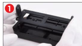
Align the base plate with hole position
