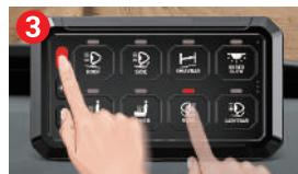
Press the button you want to set (you can choose between 8 or 12 buttons for Strobe Mode), then press the ON/OFF button to confirm, now the setting is successful
