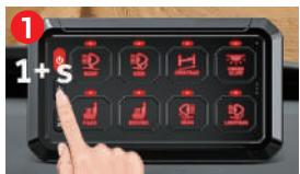
Long press the brightness adjustment button for 1 second, and the **red backlight flashes** (note: this is the Momentary setting state, please refer to its specific steps)
