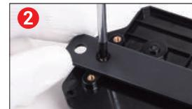
Tighten the flat head screws
