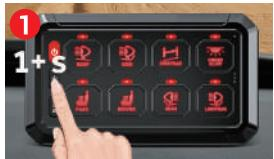
Long press the brightness adjustment button for 1 second.
