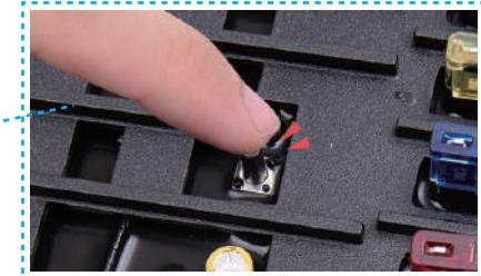
Power on the Control Box, press and hold the **pairing button**.
