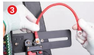
Connect circuit breaker to positive terminal of battery
