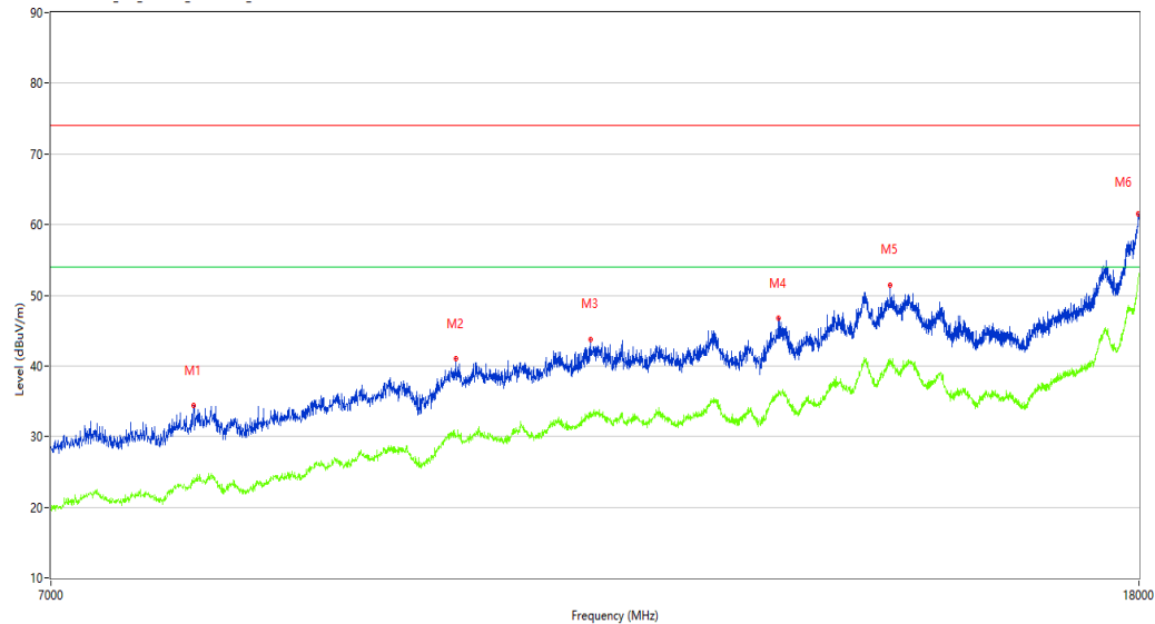
REmission Test case_FCC_Part 15C_FCC 15.247_7GHz-18GHz
