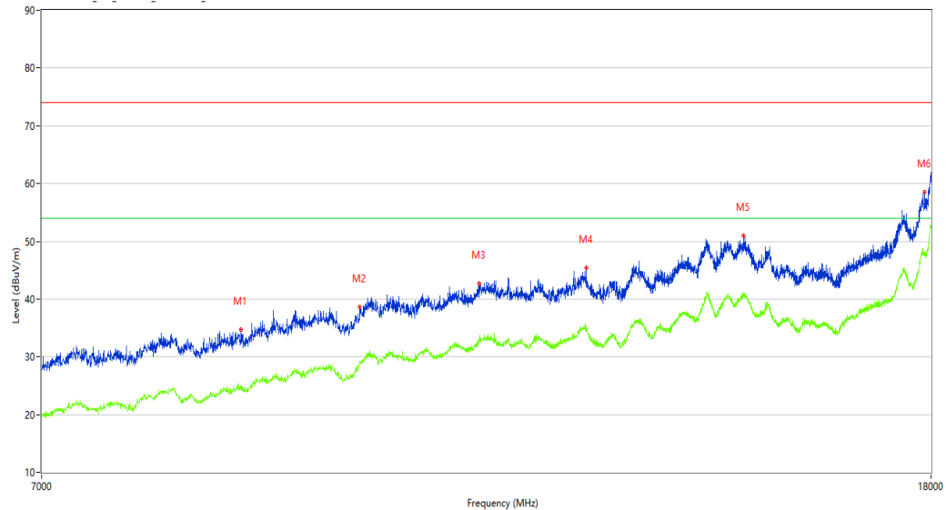
REmission Test case_FCC_Part 15C_FCC 15.247_7GHz-18GHz
