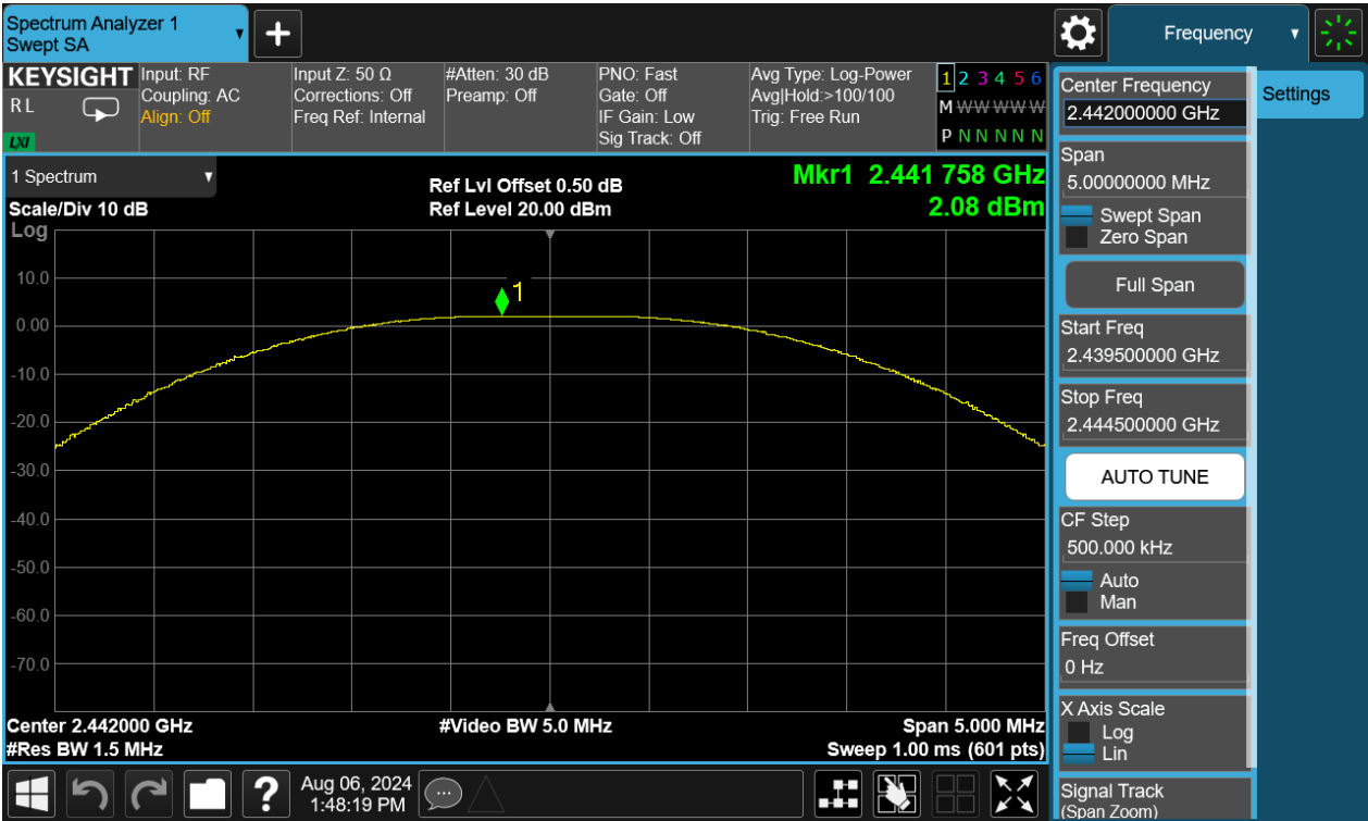
Figure 2: Peak Output Power, 2442MHz
