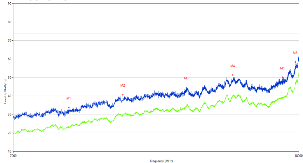
REmission Test case_FCC_Part 15C_FCC 15.247_7GHz-18GHz
