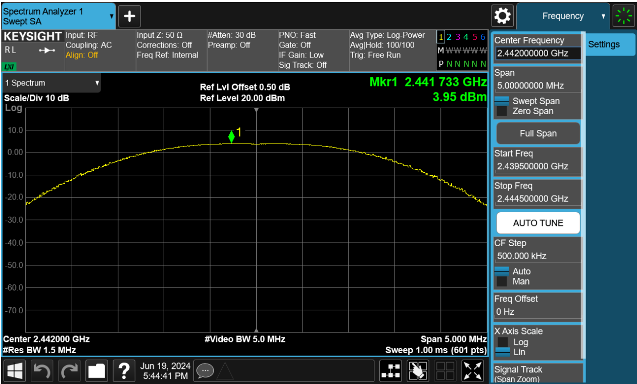
Figure 2: Peak Output Power, 2442MHz
