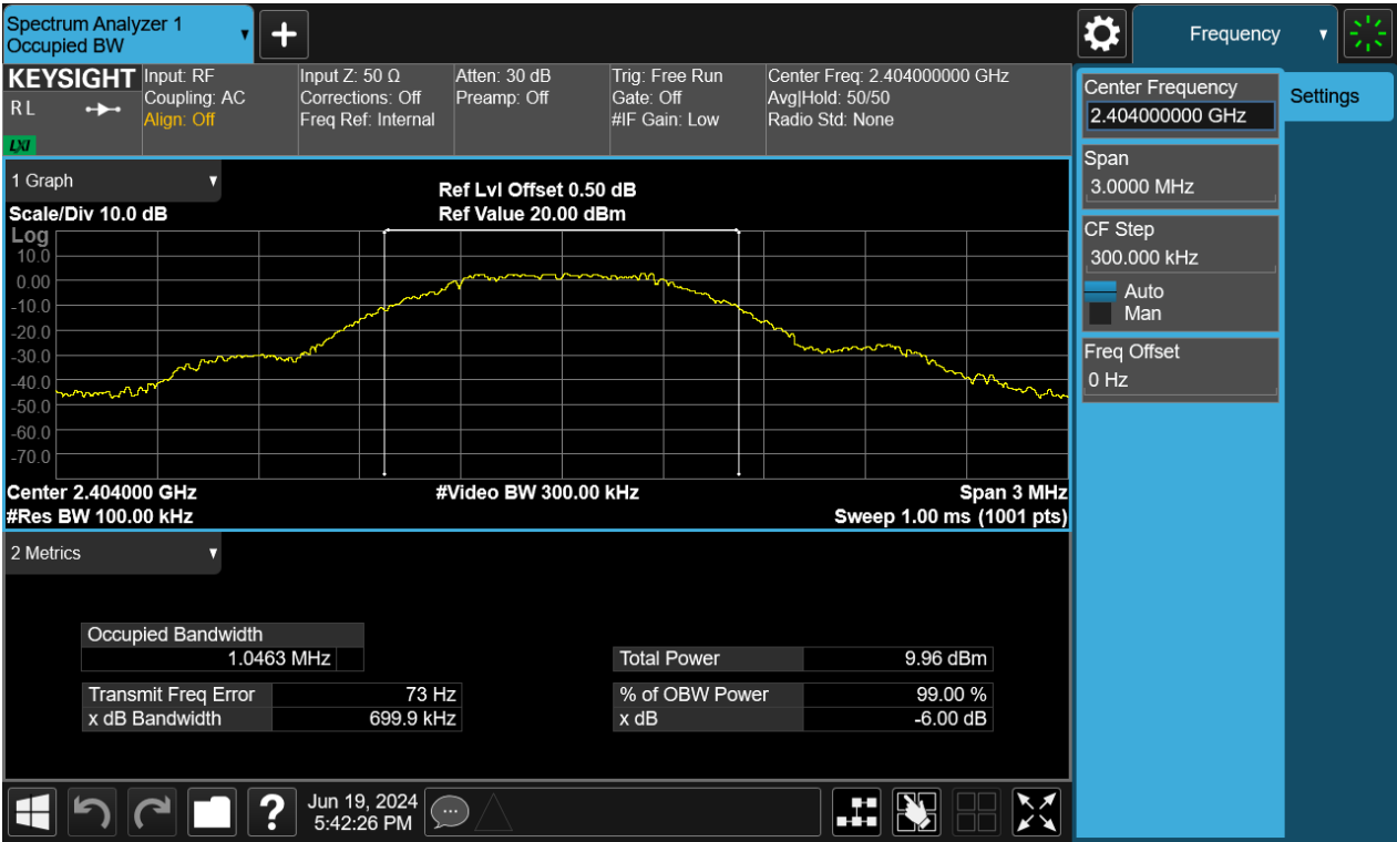
Figure 5: 6dB Bandwidth, 2442MHz
