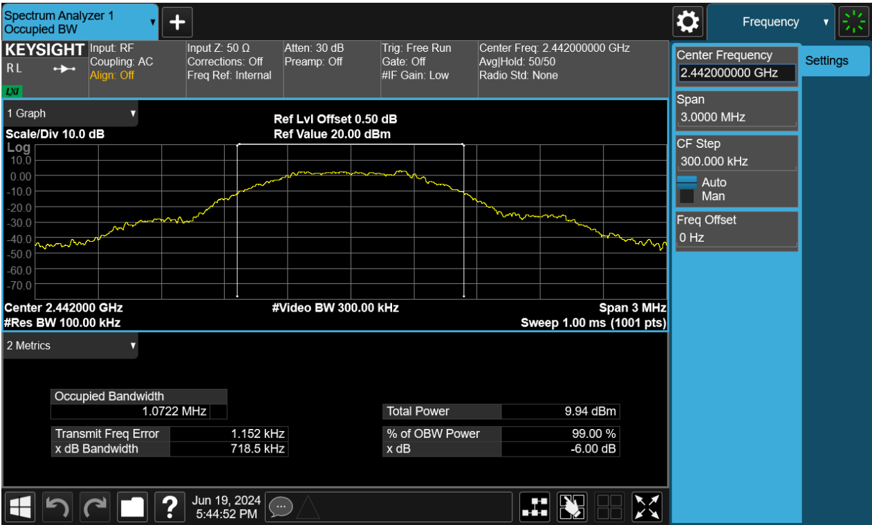
Figure 5: 6dB Bandwidth, 2442MHz
