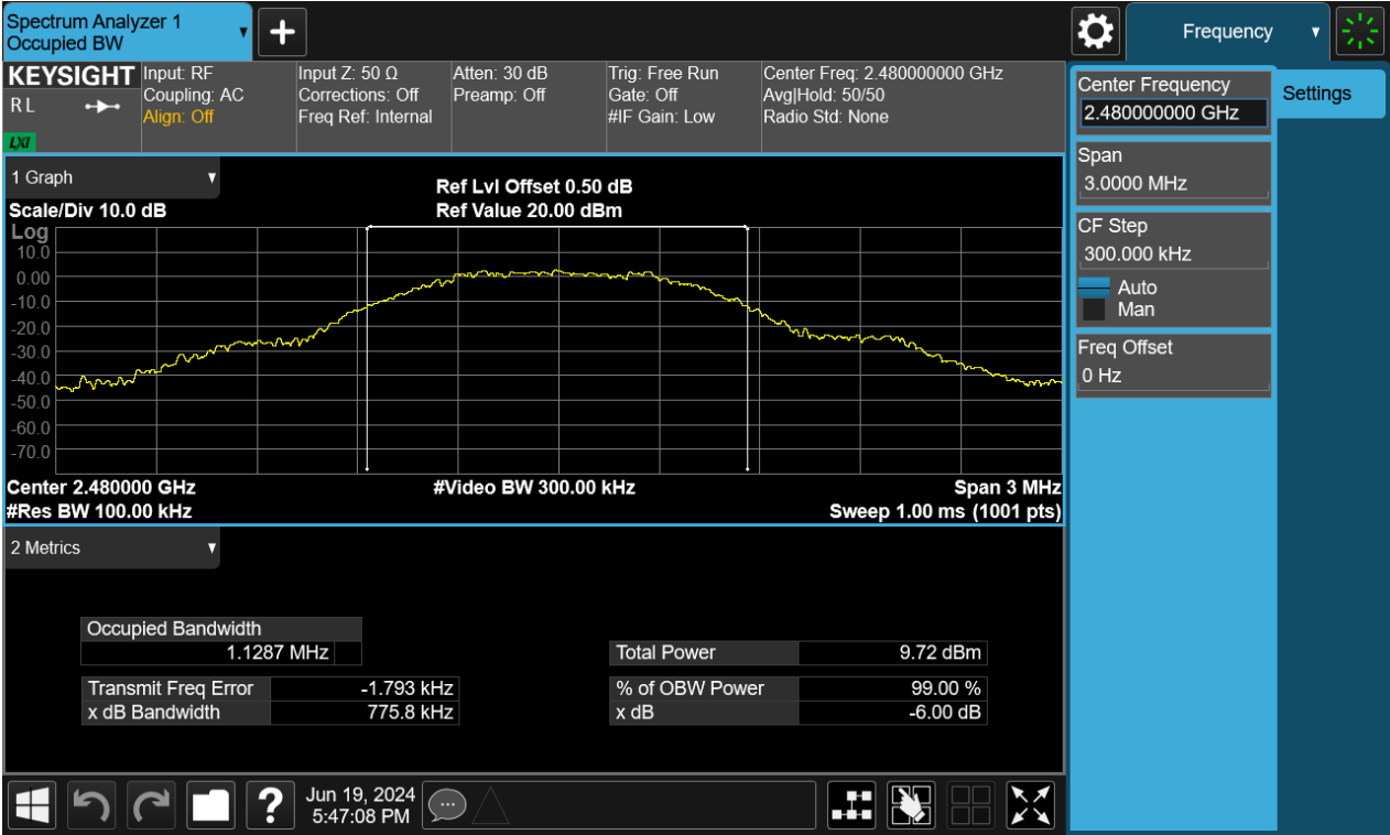
Figure 6: 6dB Bandwidth, 2480MHz
