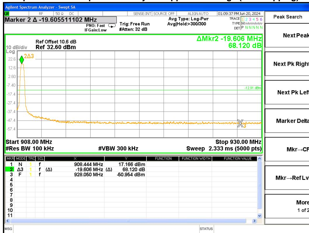
Screen Capture from the spectrum analyzer: Lower Band Edge (Hopping)
