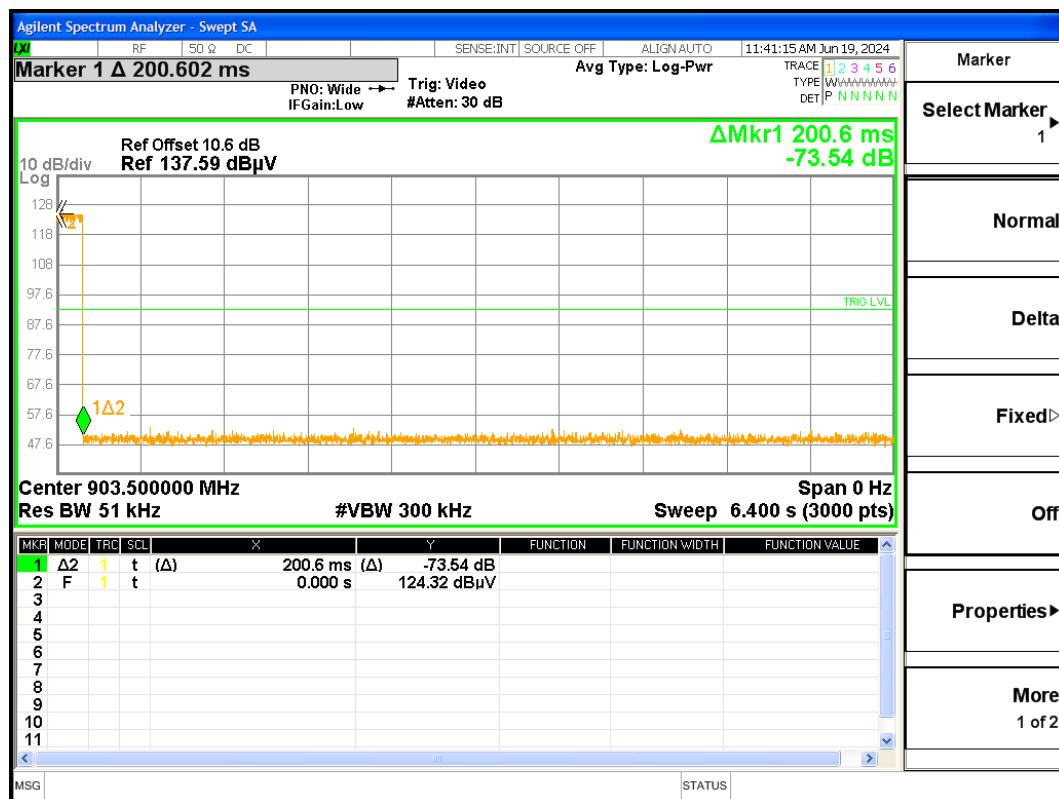
Screen Capture from the spectrum analyzer: sweep Time in 6.4 Sec 2<sup>nd</sup> Segment
