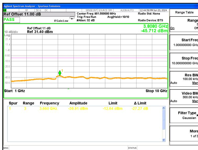
**MID Channel (Corrected Output Power: 17.3 dBm)**
