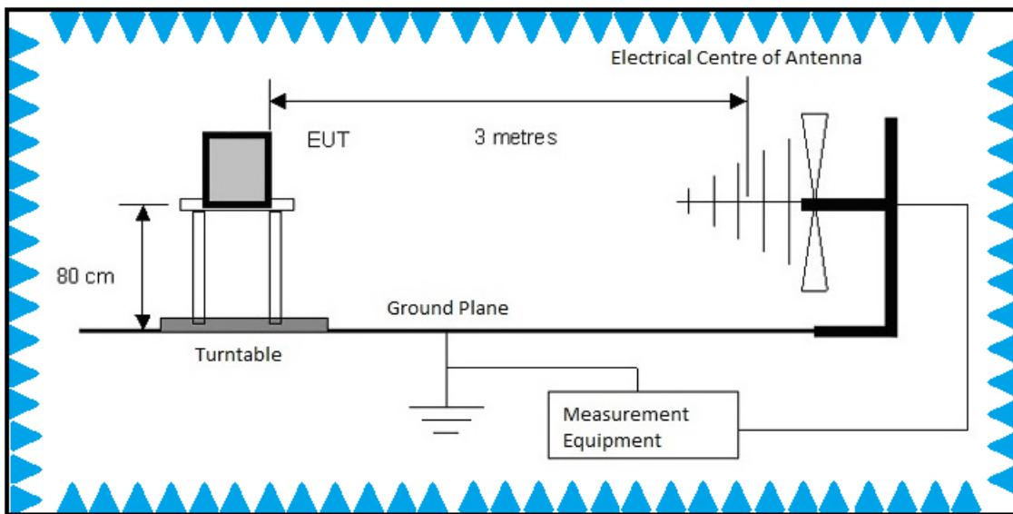
**Test setup diagram for Radiated Spurious Emissions testing (above 1GHz):**
