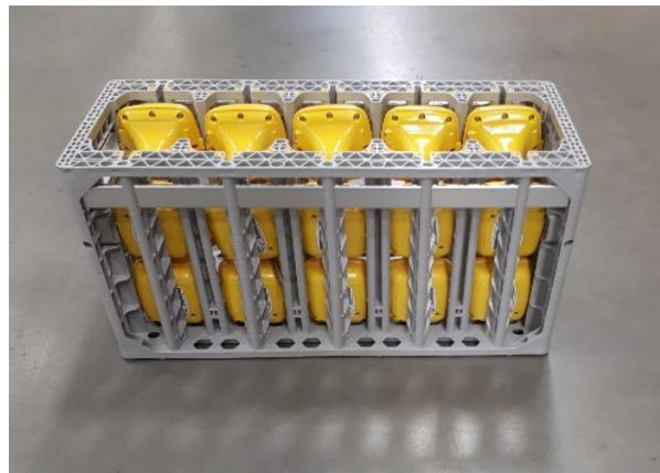
As in the picture below, where a user or shipper handler may mistakenly turn the container on its side. This would result in half the Nodes in “normal operating mode” to be in a “ON” setting and searching for GPS trying to get ready for recording and consuming Battery
