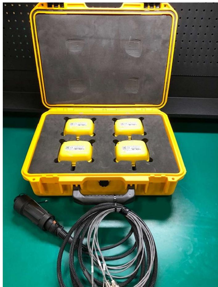
Included with the Quantum Aux Box Kit are 4 Quantum Nodes specially adapted to enable external connection of signals. They have a 2 pin Lemo connector
