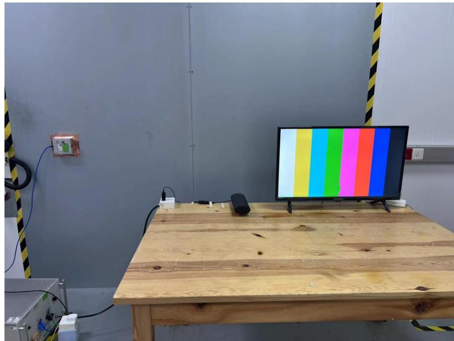
**Set-up for Radiated Emission (RE), Below 1GHz**
