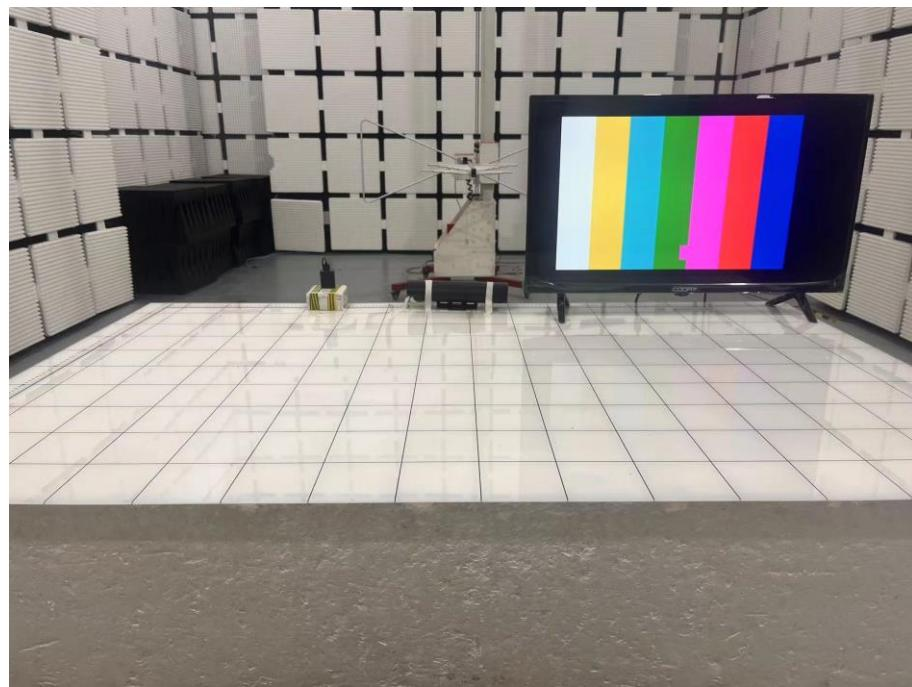
**Set-up for Radiated Emission (RE), Above 1GHz**
