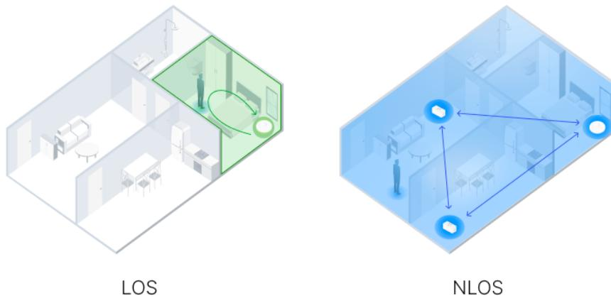
In LOS, the WiDAR Sensor can cover a room by itself without adding any other nami devices to the zone. It can cover up to 25m<sup>2</sup> / 270 sq ft. In NLOS, the WiDAR Sensor contributes to the motion-sensing mesh of its zone along with other nami devices.
