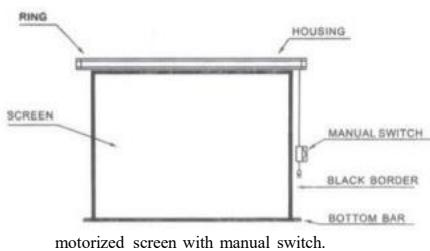
motorized screen with manual switch.
