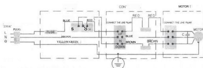
If the motorized screen work with remote control, please refer to the diagram below for electrical connection.
