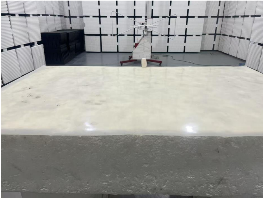
Set-up for Radiated Spurious Emission, Above 1GHz
