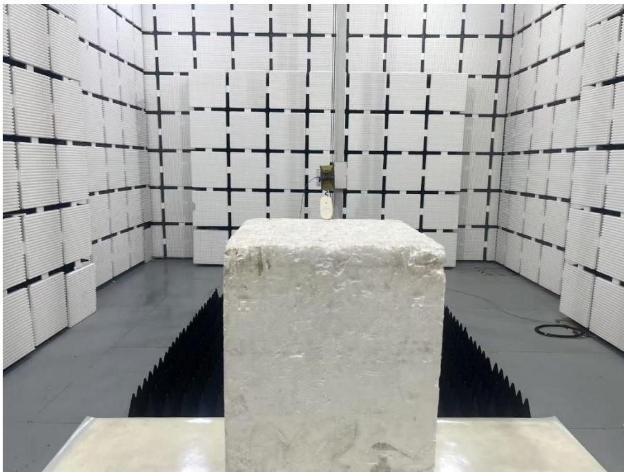
Set-up for Radiated Spurious Emission, Above 1GHz
