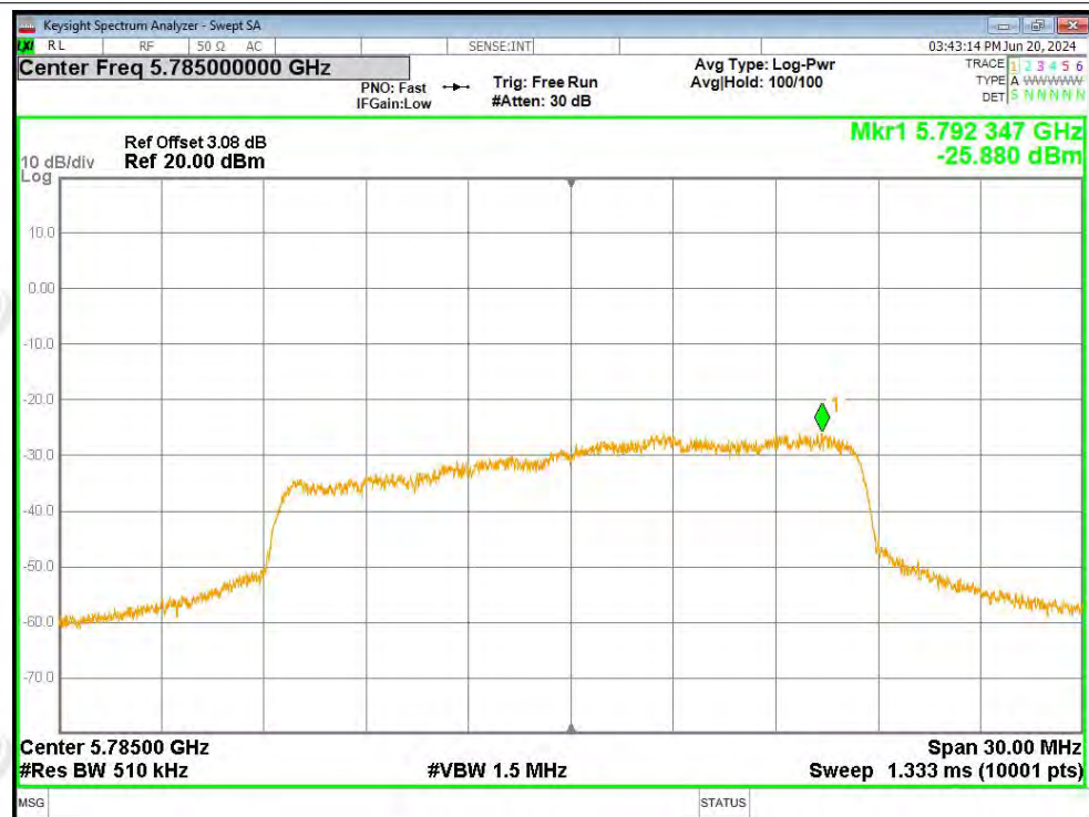
PSD NVNT a 5825MHz Ant2
