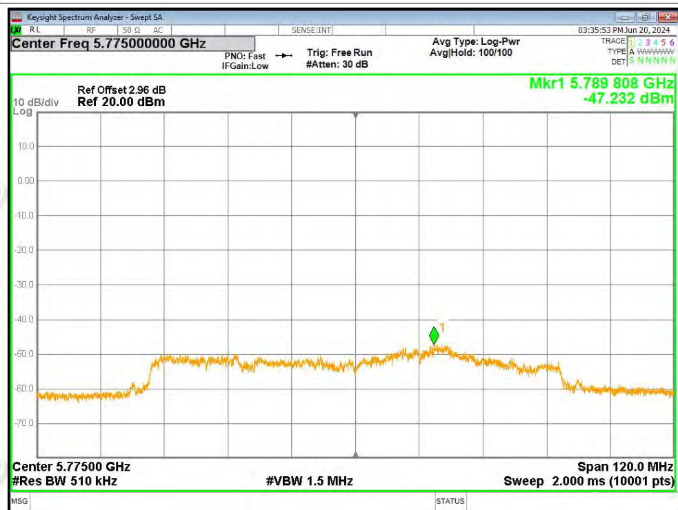
PSD NVNT ac80 5775MHz Ant2
