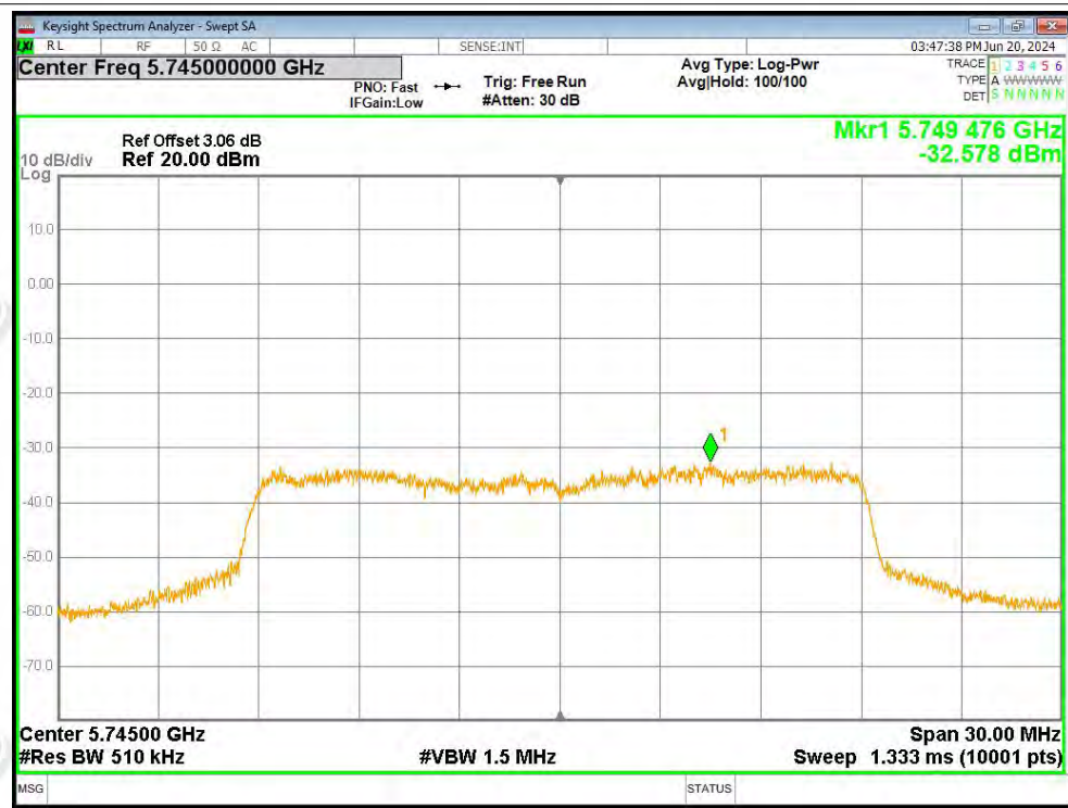
PSD NVNT n20 5745MHz Ant2
