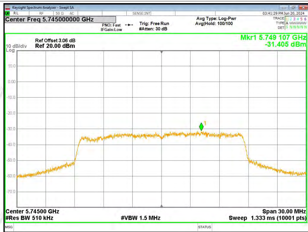
PSD NVNT a 5745MHz Ant2
