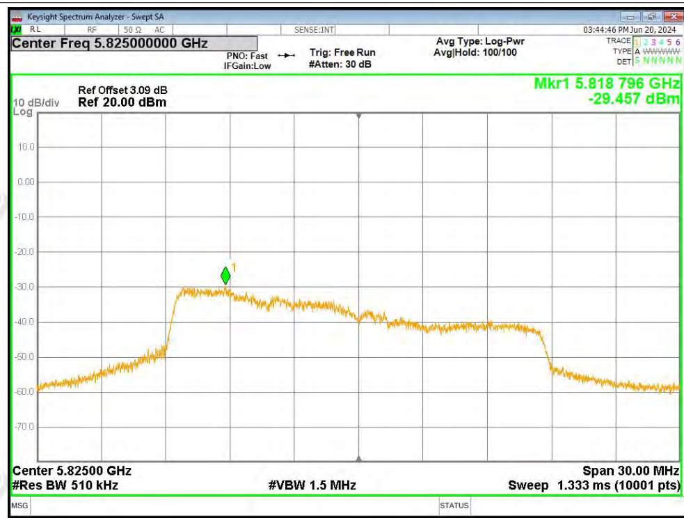
PSD NVNT a 5825MHz Ant2
