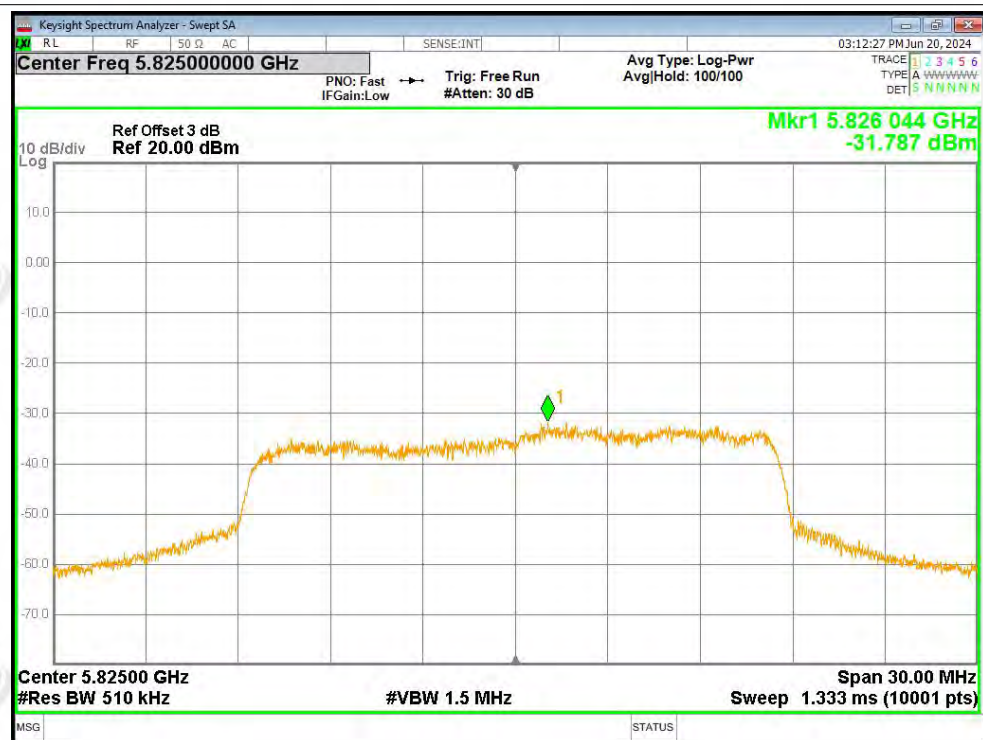
PSD NVNT a 5745MHz Ant2
