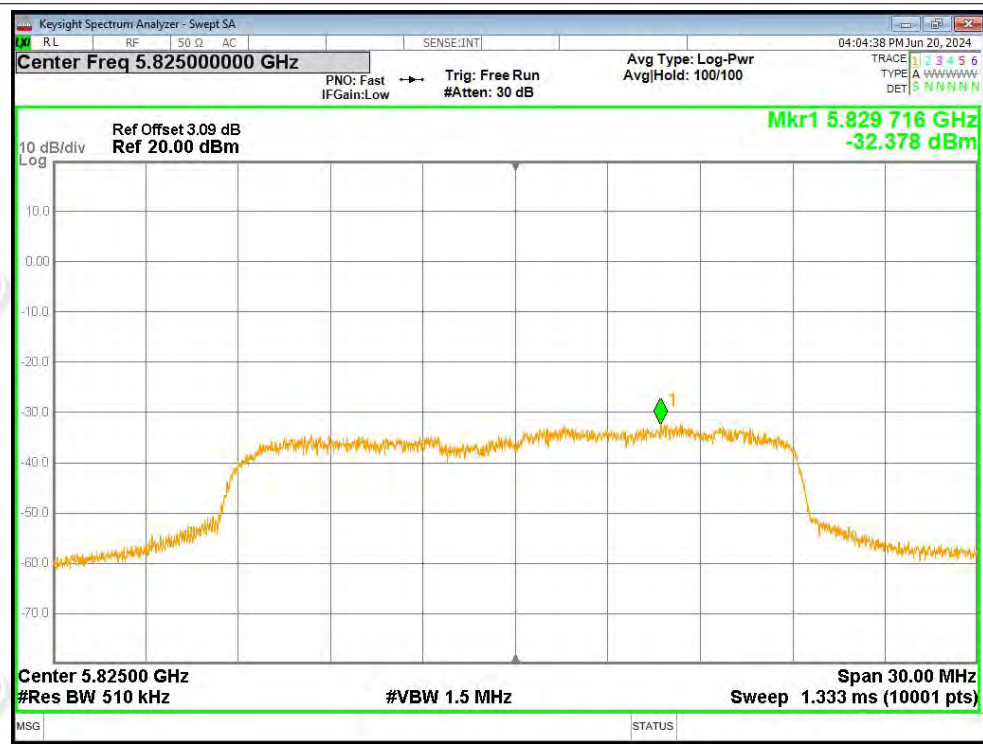
PSD NVNT ac20 5825MHz Ant2
