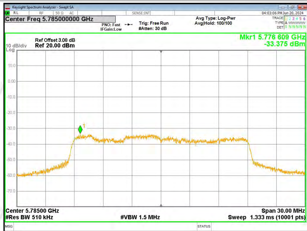
PSD NVNT ac20 5825MHz Ant2
