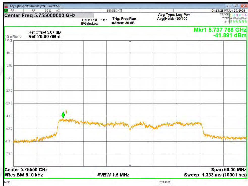
PSD NVNT ac40 5795MHz Ant2
