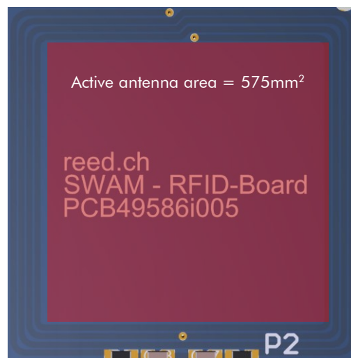
Figure 5: RFID Read Writer mechanical dimensions antenna
