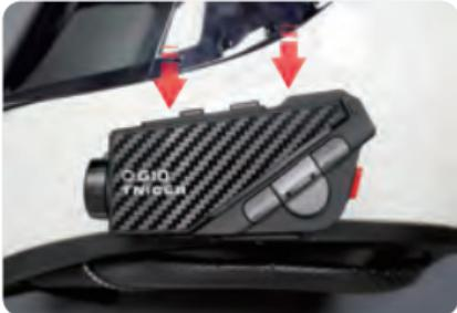
④ Push the device toward the bottom of the helmet and snap it into the rotating cradle, the installation is complete.
