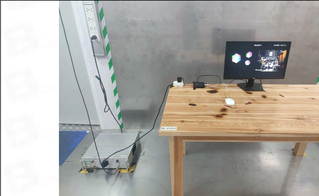
Conducted Emission at AC power line
