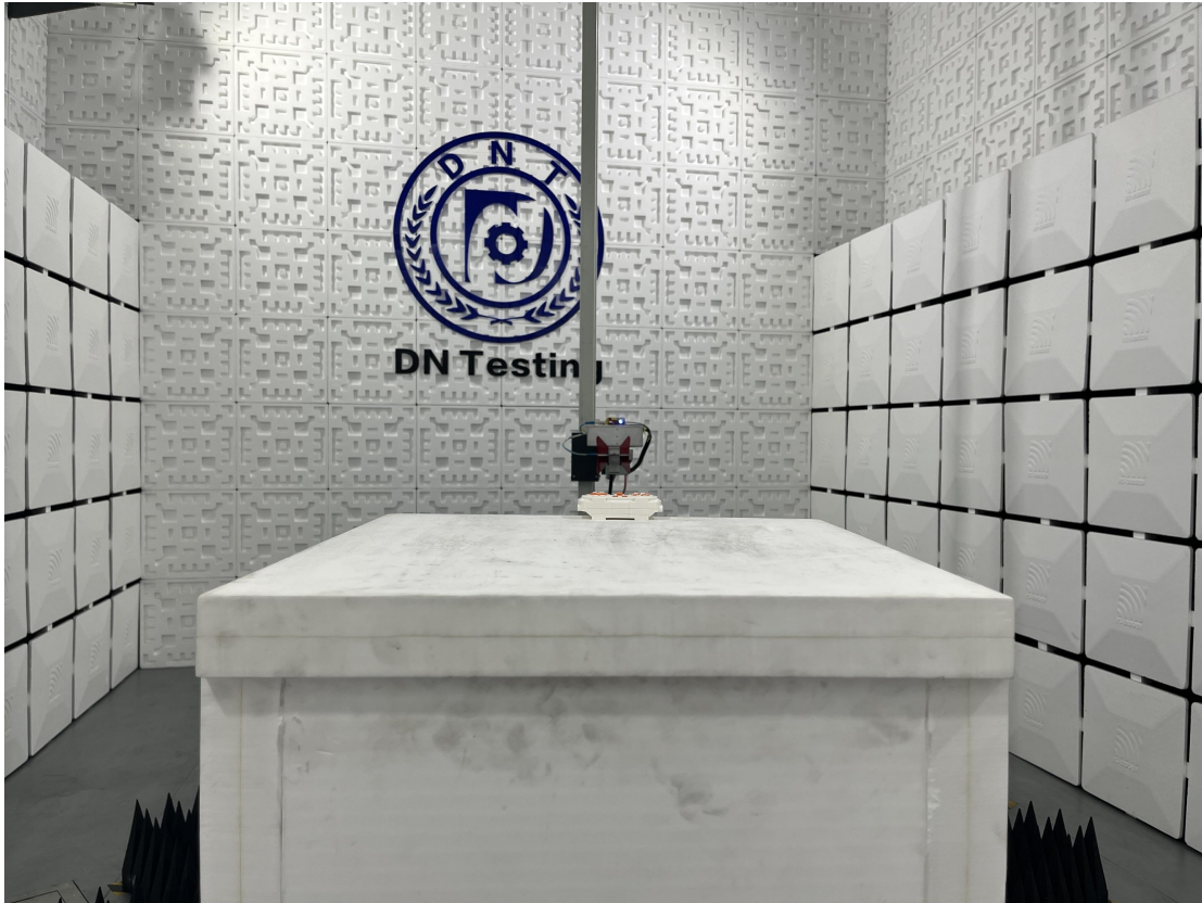
Radiated Emission Test View|(Above 1G)
