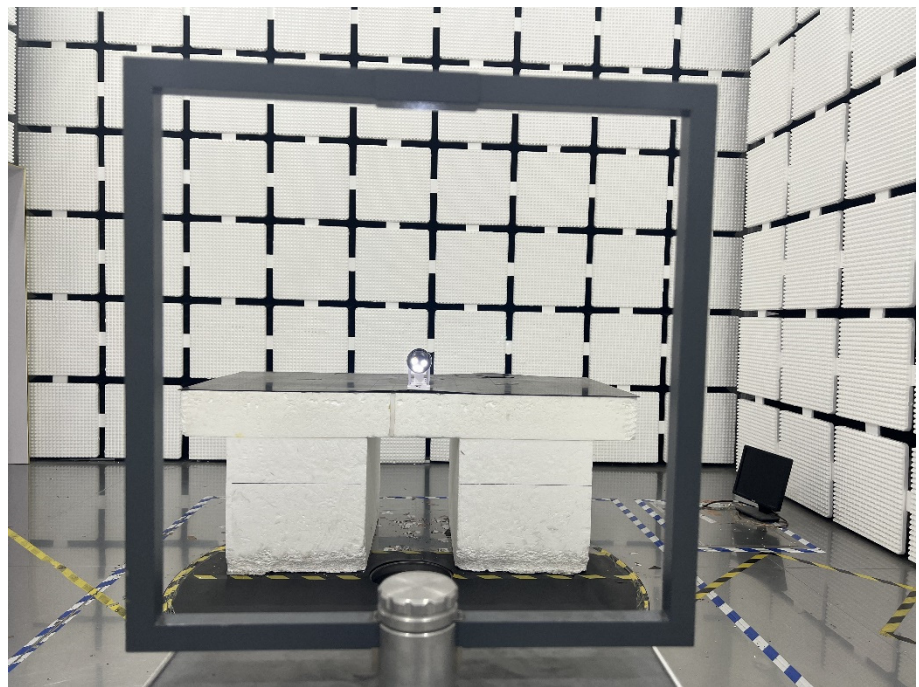
Radiation Emission Test Setup (Below 30MHz)
