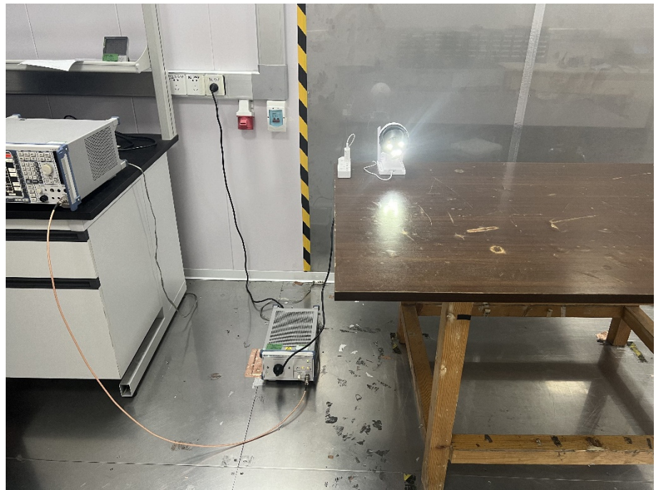
Conducted Emission Test Setup
