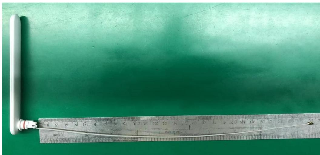
**The physical product has a 1.13mm wire with a length of 280mm.**
