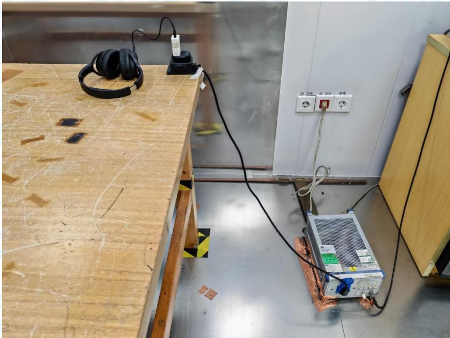
Photo of Setup for Radiated Emission (30MHz~1GHz)
