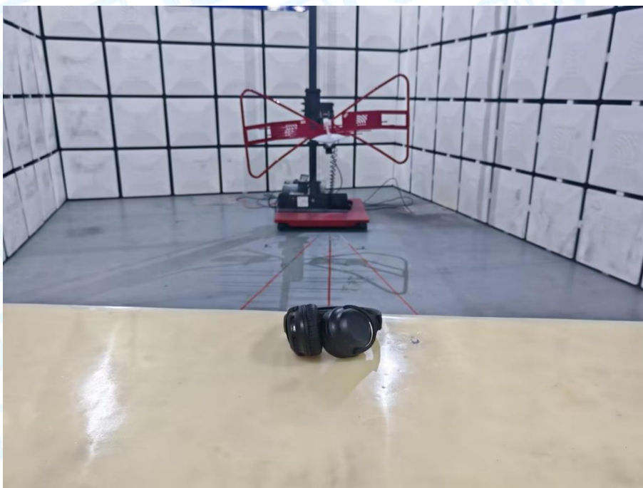
Photo of Setup for Radiated Emission (30MHz~1GHz)
