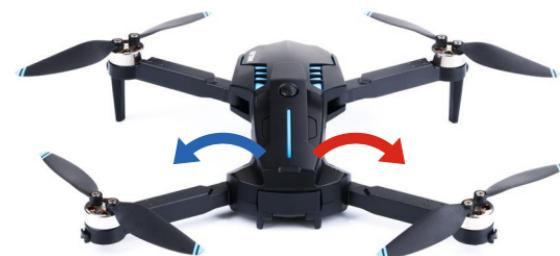
1. After the drone reaches a height of 10 feet/3 meters or more, press the roll button, and the drone will enter a standby state for rolling.
