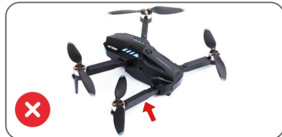
3. Check and Address Propeller Issues: If the propellers are stuck together, be sure to manually separate them promptly, as this entanglement could cause the drone to go out of control. Similarly, if any foreign objects are entangling the propellers, immediately untangle and clear them, as these objects would affect the normal rotation of the propellers and could result in the drone losing control.
