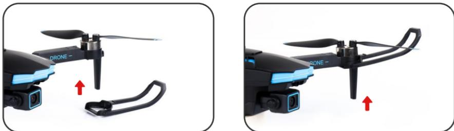
1. Locate the mounting point: Align the propeller guards with the drone's arm for mounting (Illustration 1) and press until it's in place.
