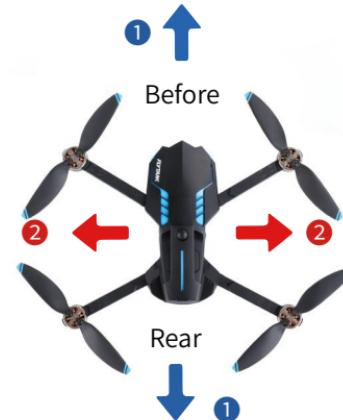
1. If the drone exhibits unstable flight behaviors, such as drifting in a certain direction or spinning in mid-air, the trim function can be used to correct it.
