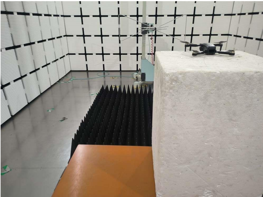
Radiated Emission Test View Above 1GHz
