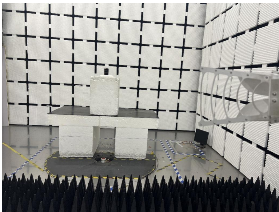
Radiation Emission Test Setup (1GHz to18GHz)
