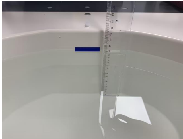
Liquid Height for Head/Body SAR
