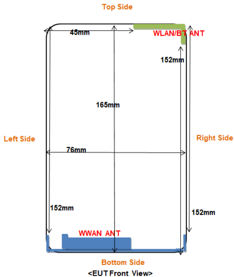
Block Diagram for EUT Antenna Position
