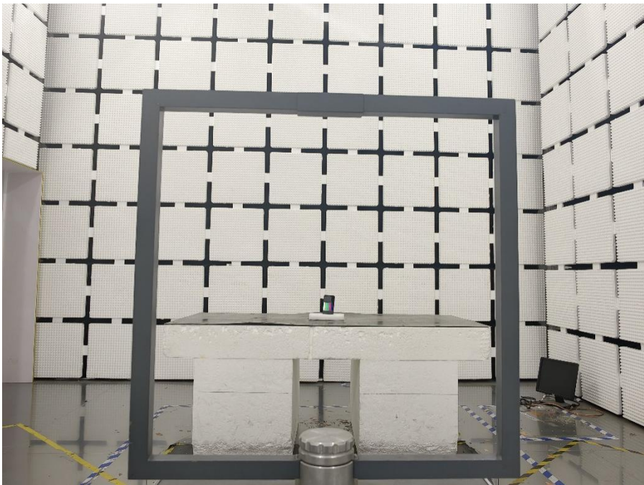
Radiation Emission Test Setup (Below 30MHz)
