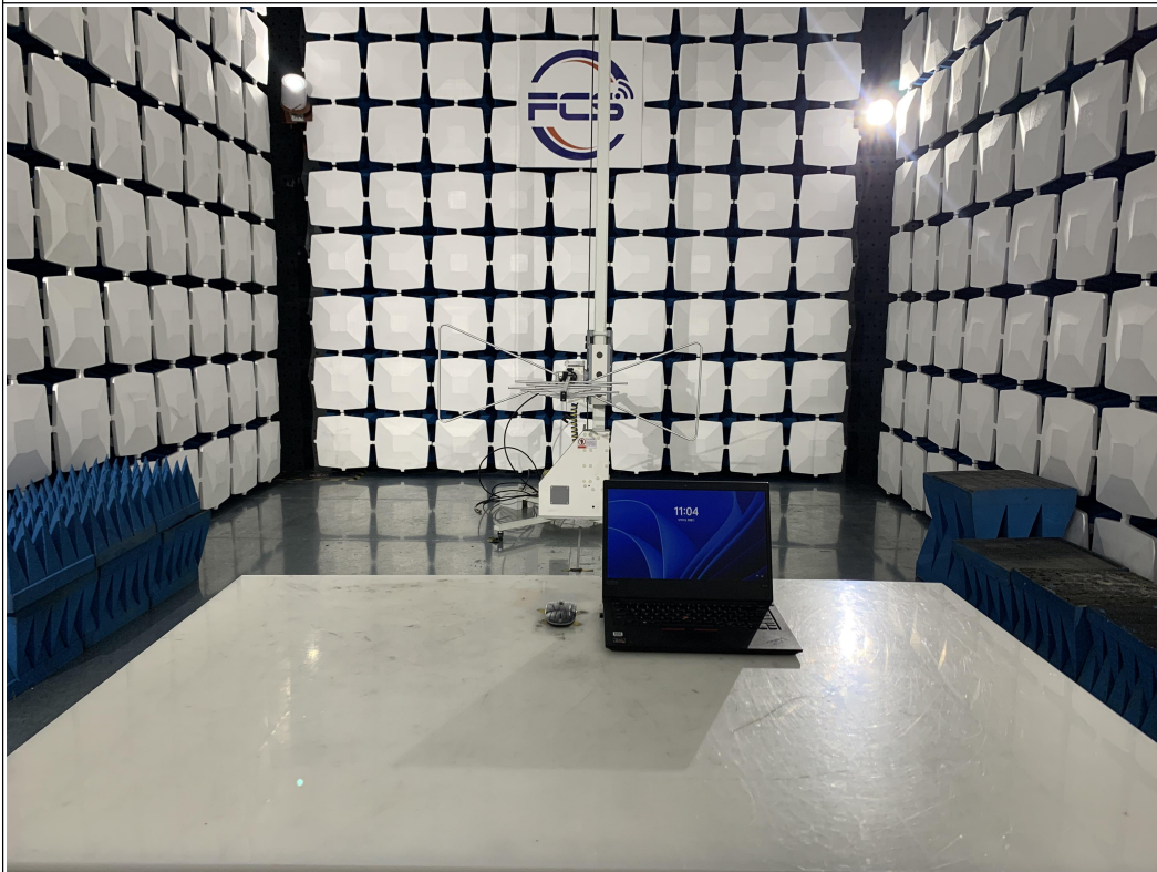
Above 1GHz for radiated emission test setup
