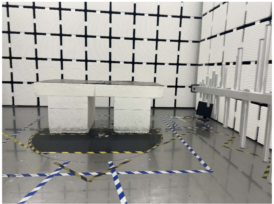
Radiation Emission Test Setup (30MHz to 1GHz)
