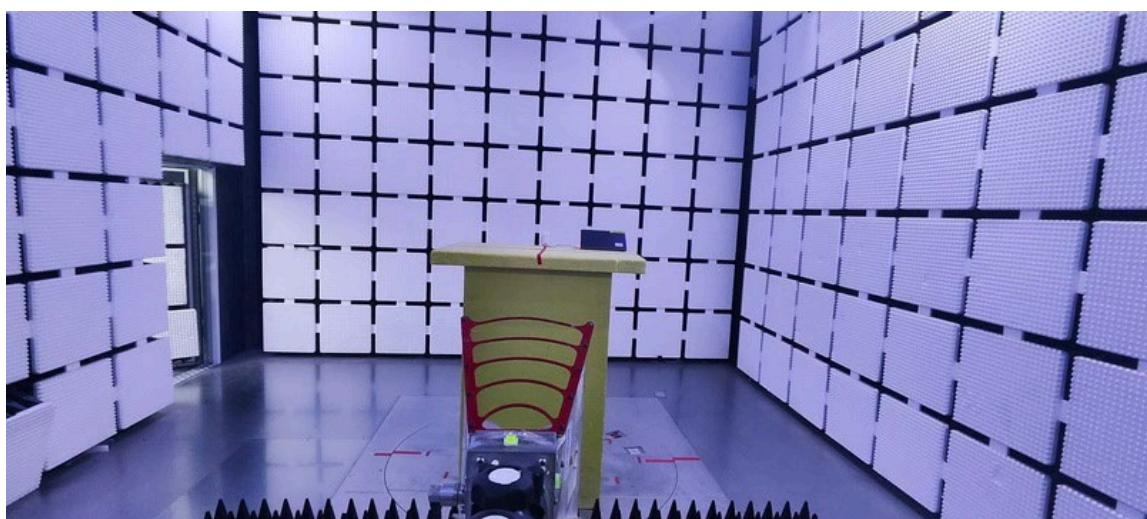
**Radiated Emissions Test Photos****Harmonic(18 GHz to 26.5 GHz)**
