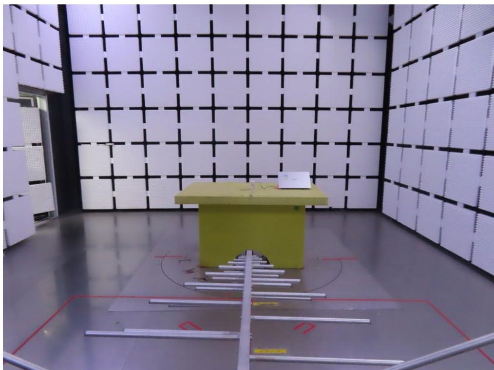
**Radiated Emissions Test Photos****Band edge & Harmonic(1 GHz to 18 GHz)**
