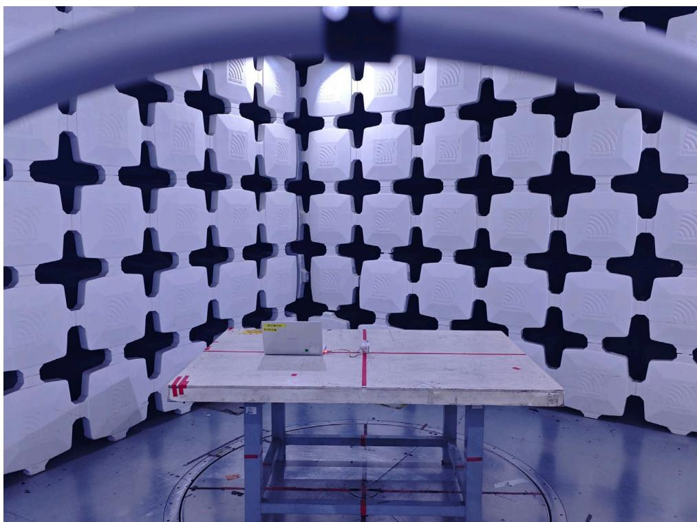
**Radiated Emissions Test Photos****30 MHz to 1000 MHz**
