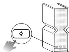
2. Within 2 minutes, press the WPS button on the extender for 1 second, and the LED starts blinking. Wait for the LED, 2.4GHz LED, and 5GHz LED to turn solid blue, indicating a successful connection.
