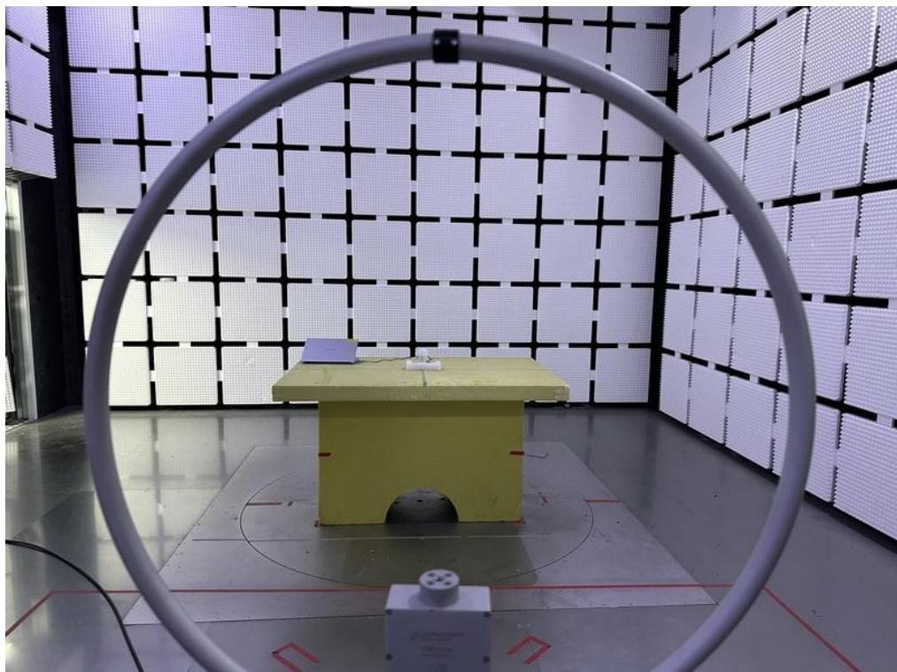
**Radiated Emissions Test Photos****30 MHz to 1 GHz**
