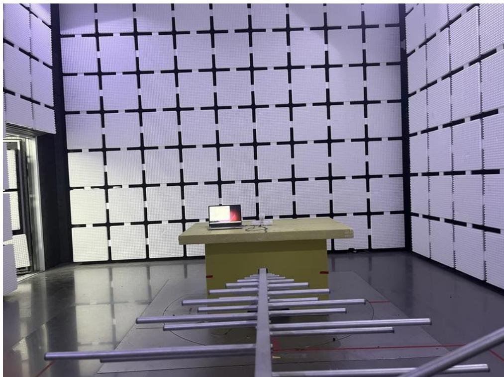
**Radiated Emissions Test Photos****Band edge & Harmonic(1 GHz to 18 GHz)**
