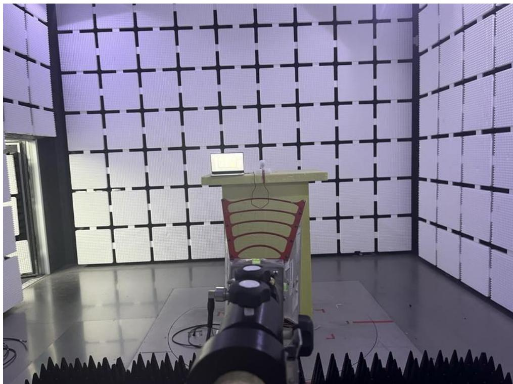
**Radiated Emissions Test Photos****Harmonic(18 GHz to 26.5 GHz)**
